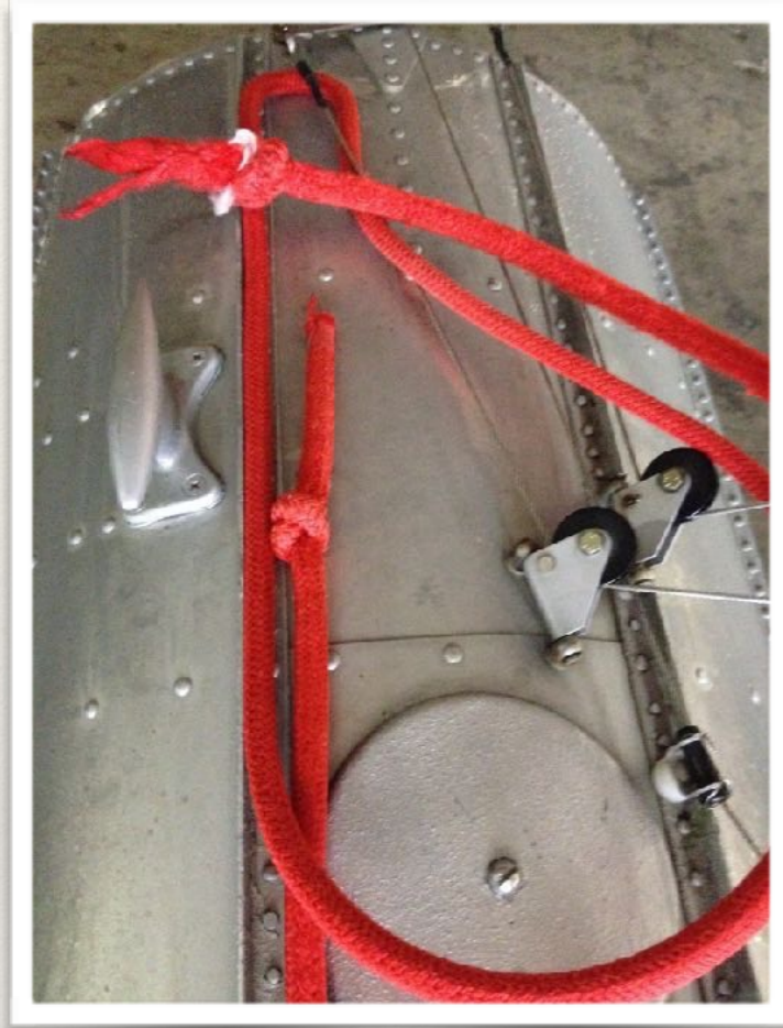
Too long - interferes with cables and water rudder
