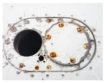
The key to preventing corrosion on metal aircraft is to shield the metal from electrolytes. There are several ways in which this can be accomplished. The FAA advisory circular FAA AC 43.13-1B - ACCEPTABLE METHODS, TECHNIQUES, AND PRACTICES — AIRCRAFT INSPECTION AND REPAIR recommends aircraft be treated with Zinc chromate primer, par-al-ketone, non-water soluble grease, or comparable materials when used as seaplanes.
