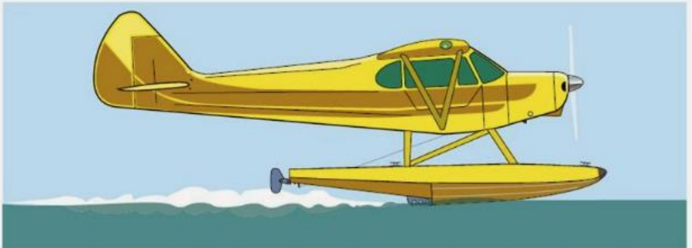
Figure 4-7. On the step. The attitude is nearly level, and the weight of the seaplane is supported mostly by hydrodynamic lift. Behind the step, the floats are essentially clear of the water.
