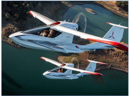
three-blade prop, Icon claims that the new E-Props propeller improves ground takeoff performance by 21%.
